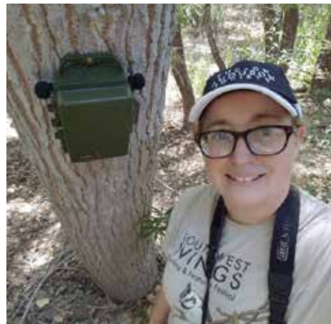
Jennie and TAS SM4 Sound recorder set up along the San Pedro River to capture diagnostic sounds of migrants and spring nesters in this habitat
